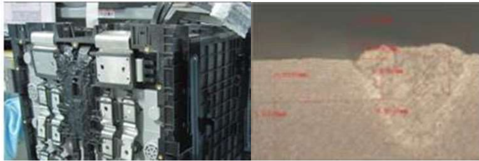
Figure 10: Laser Welding Between Batteries and Ultrasonic welding in the cell
