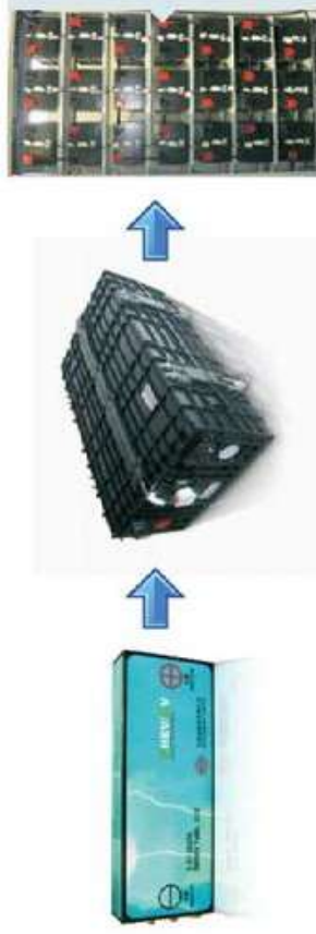
Figure 2. Battery Cell, Module, and Pack
