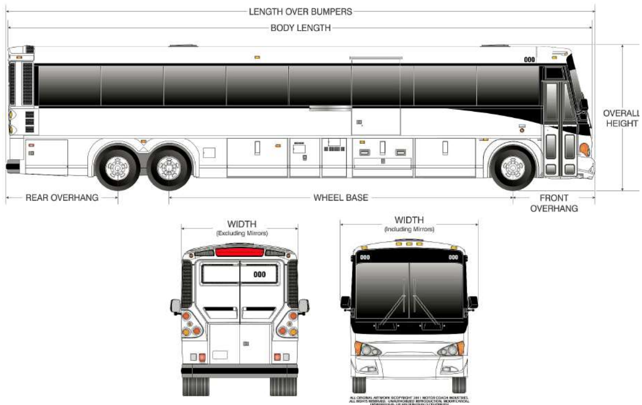
FIGURE 1 Transit Bus Exterior Dimensions
