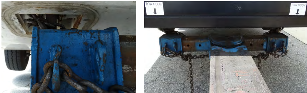
Figure 1-17. Install Tow Fork Safety Chains
