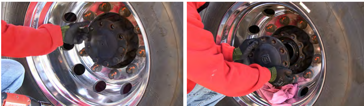
Figure 1-20. Removing the Half Shaft
