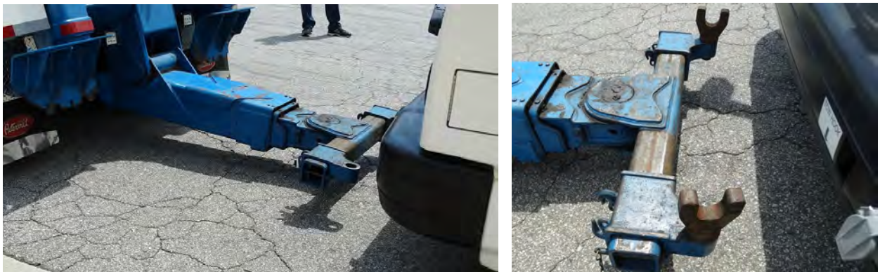
Figure 1-14. Positioning Stinger Under Front of Bus
