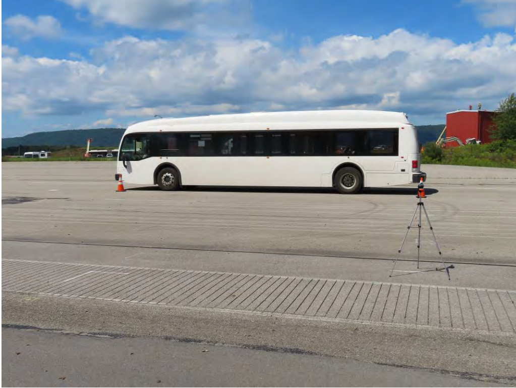
TEST BUS UNDERGOING EXTERIOR NOISE TESTING
