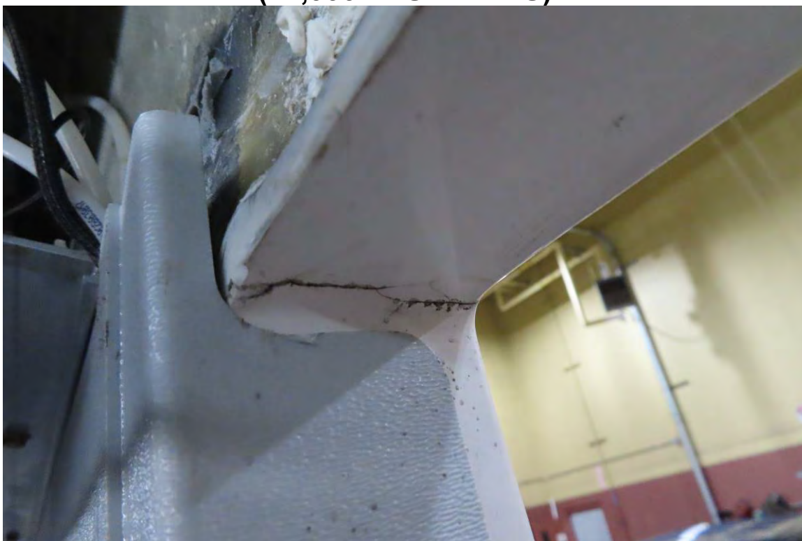
CRACKS AROUND REAR DOOR (12,999 TEST MILES)
