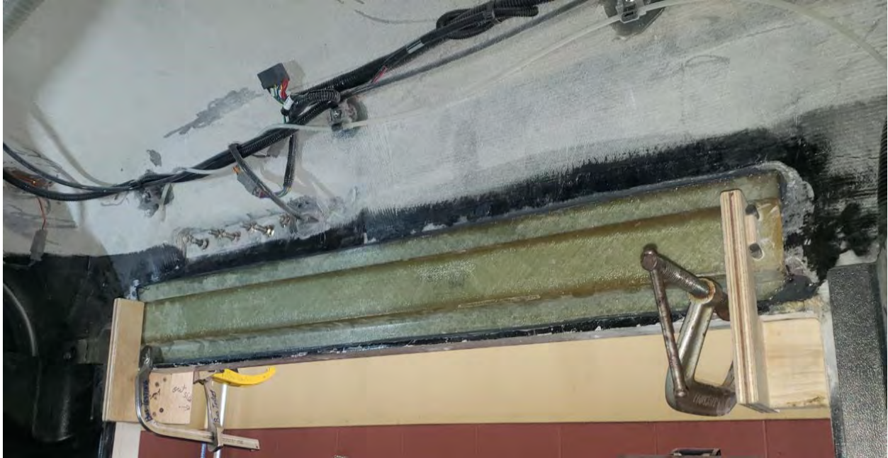
FRONT DOOR HAT BRACKET REPAIR (6,494 TEST MILES)
