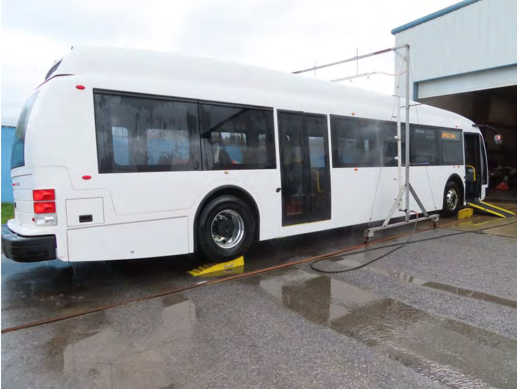
RIGHT REAR WHEEL SIX INCHES HIGHER
