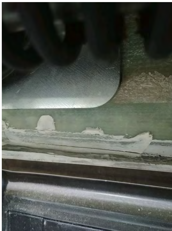
CRACKS AROUND REAR DOOR (12,999 TEST MILES)
