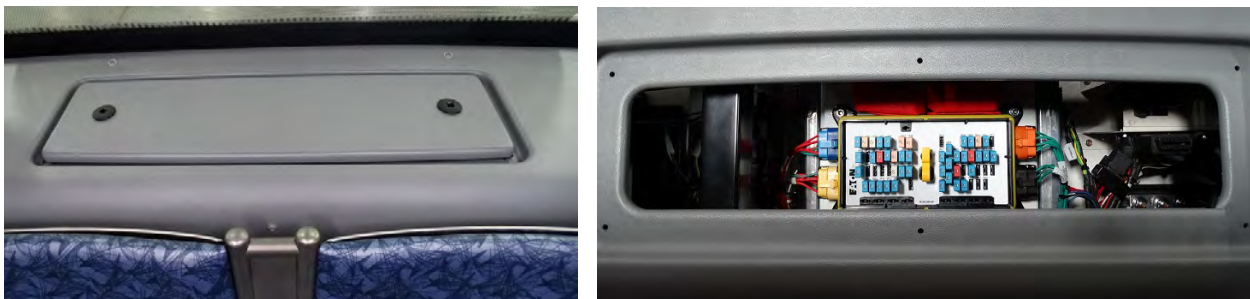
Figure 1-4. Opening the Rear Deck Access Covers
