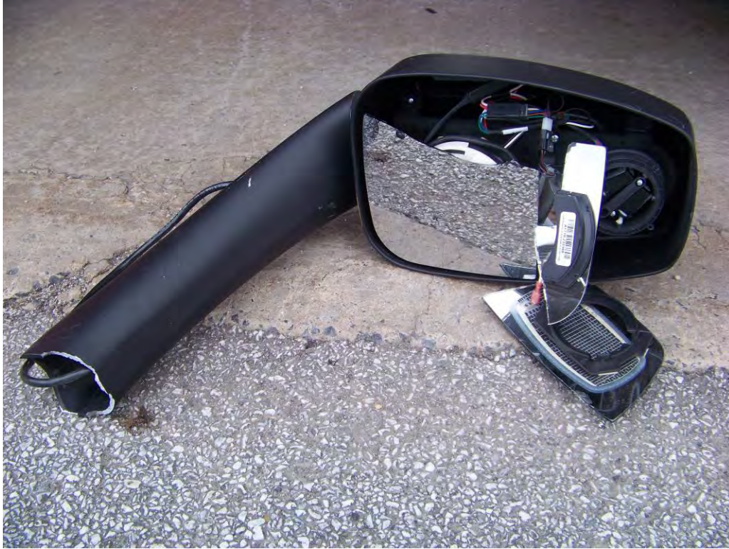
CURBSIDE MIRROR ARM SNAPPED (681 TEST MILES)
