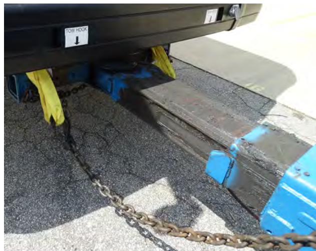
Figure 1-18. Install Tow Fork Safety Chains
