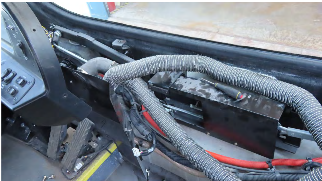
DASH PIECES REMOVED TO ACCESS WIPER MOTOR
