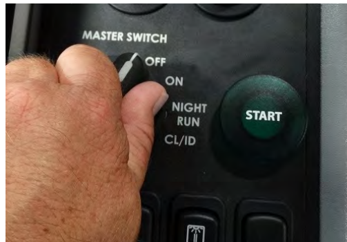
Figure 1-21. Turn ON Master Switch
