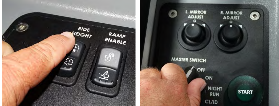
Figure 1-2. Maximize Ride Height and Turn OFF Master Switch
