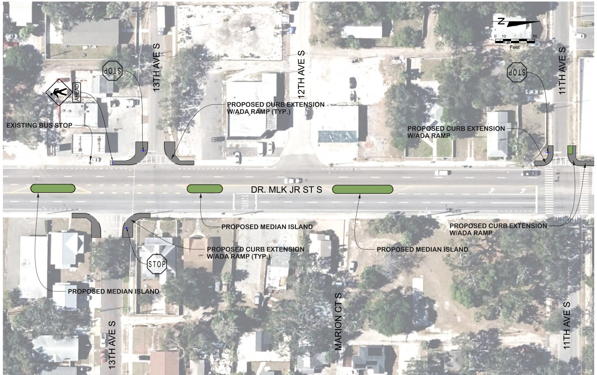
Figure 18. Dr. Martin Luther King, Jr. Street S Concept - 13th Avenue S to 11th Avenue S
